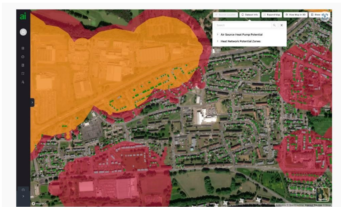
Heat Network Potential Zones from the Scottish national assessment overlaid with a desktop assessment of domestic air Source heat pump potential produced by Advanced Infrastructure
