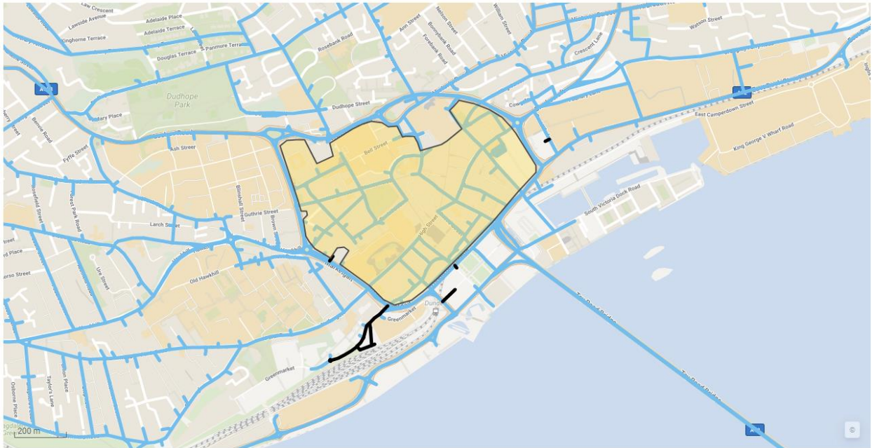
Figure 11 – Roads highlighted in black are predicted to see an increase in NO x emissions of over 40%, with an average of 125%.
