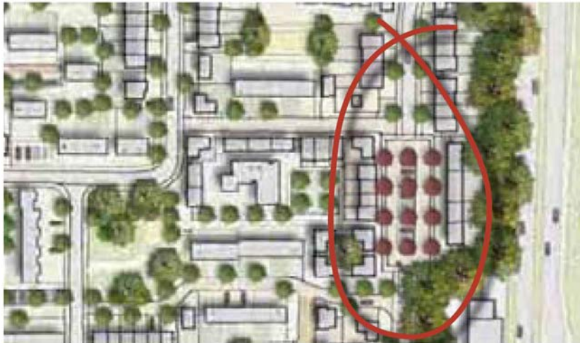
We propose to introduce traffic calming on Hebrides drive at the existing shops. This could be by making a central island with trees and parking, and diverting the traffic around this.
