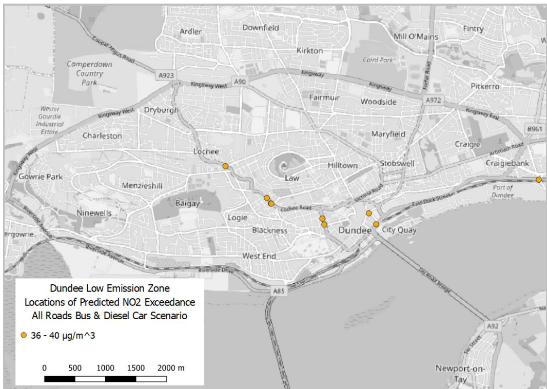
Figure 3.5 : Locations of predicted NO 2 greater than 36 µg/m 3 – Bus & diesel car
