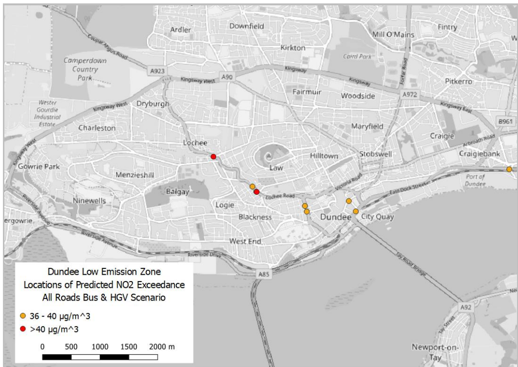
Figure 3.6 : Locations of predicted NO 2 greater than 36 µg/m 3 – Bus & HGV
