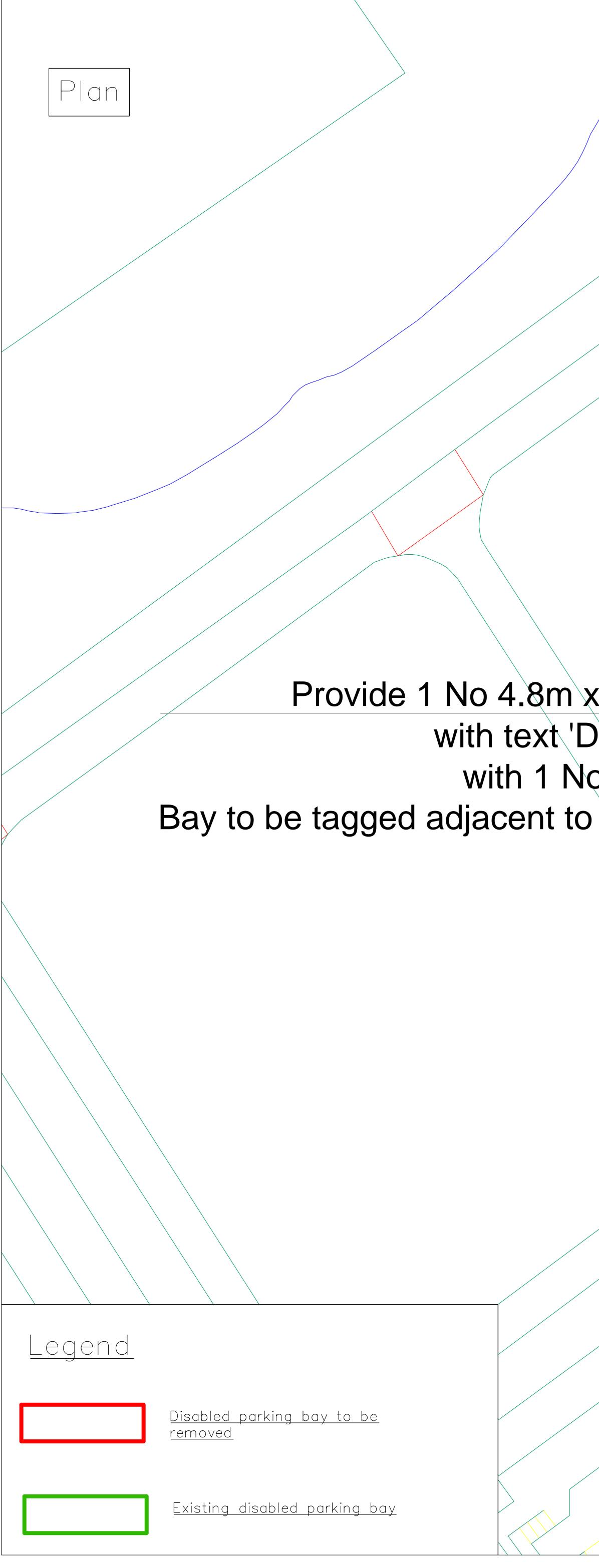
Provide 1 No 4.8m x 2.4m disabled bay as shown with text 'DISABLED' on the carriageway with 1 No Infomaster bollard as shown. Bay to be tagged adjacent to existing disabled parking bay.
