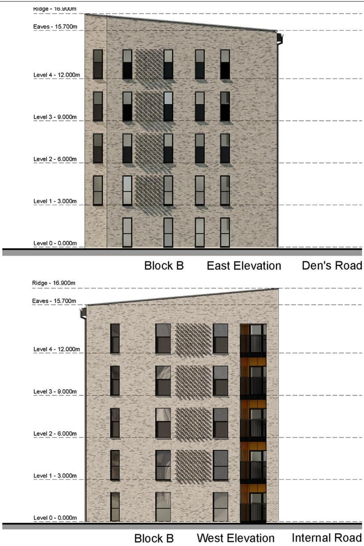
Figure 5- Block B elevations
