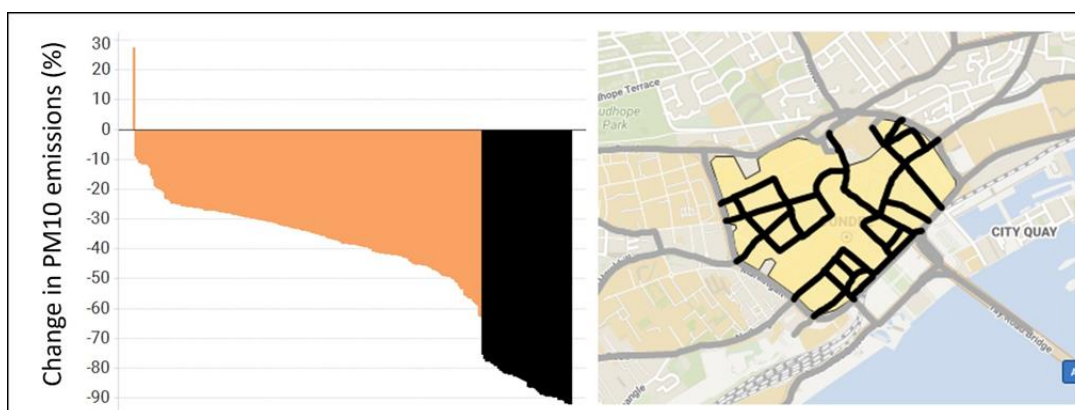
Figure 17: Ranked changes in PM 10 emissions (%) on all roads. The greatest reductions occur inside the LEZ as highlighted in black.
