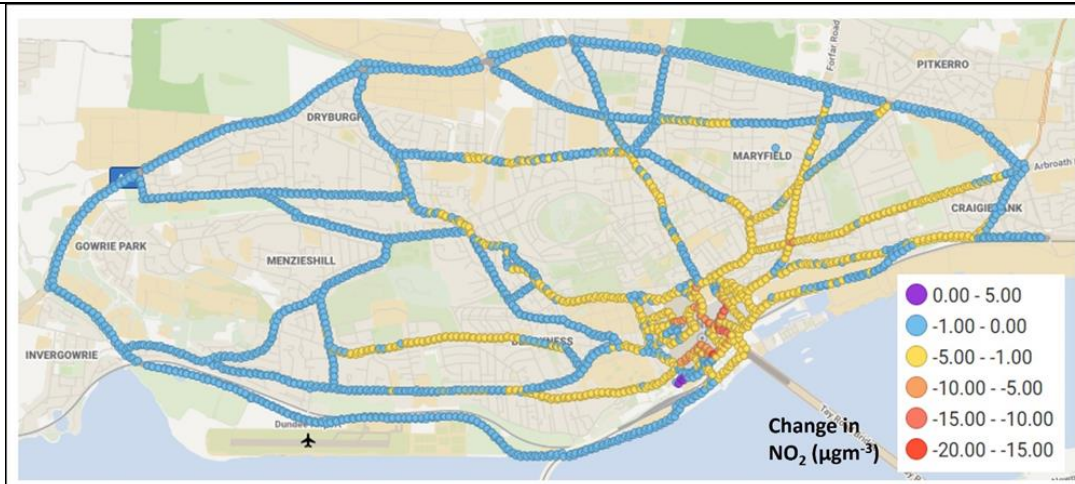
Figure 16: Relative changes in NO 2 concentration between Reference and LEZ cases across the entire model domain.
