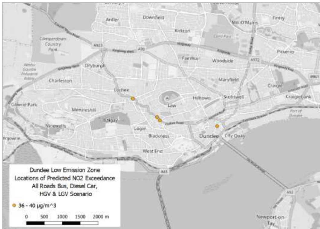
Figure 3.8 : Locations of predicted NO 2 greater than 36 µg/m 3 – Bus, diesel car, HGV & LGV
