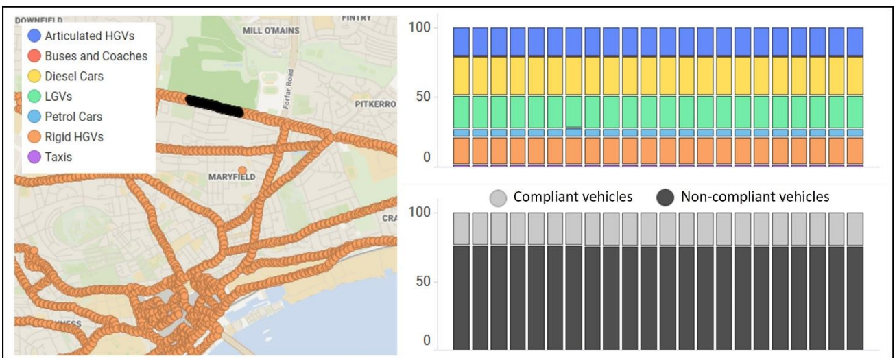
Figure 23: The contribution to modelled NO x concentrations from different types of vehicle, at roadside points on the Kingsway.
